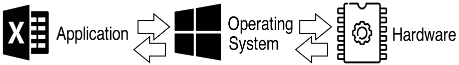
Figure 1.11: Applications control the operating system to control the hardware.
